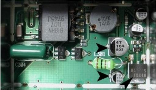
This transistor has no way of cooling laying flat on the board. remove this at your own risk. You have to have a small tip iron and a good set of eyes and steady hands. The center leg on the transistor is cut off, this is the ground leg, and the top of the transistor is soldered to the board.
