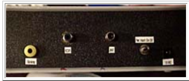
A view of the rear panel of the synchronous noise blanker. A banana jack (left) is for monitoring the blanking pulse with an oscilloscope. (Click on the picture for a larger view)
