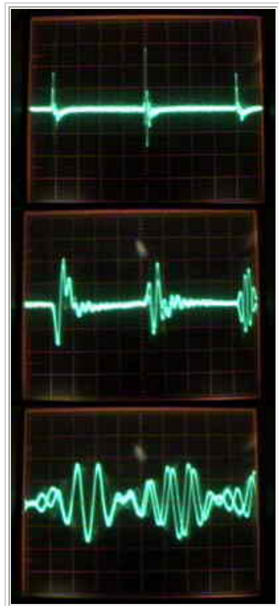
From top to bottom: Dimmer noise pulses in a 12 KHz, 2.2 KHz, and a 300 Hz filter. Note the widening of the pulses with progressively narrower filters. (Division are 2 ms)
