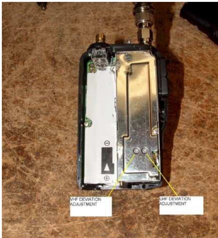
Fig. 4 Deviation adjustment for the VX-1R. VHF is on the left, UHF is on the right. Don't turn more than about 10-15 degrees CLOCKWISE to increase deviation.
